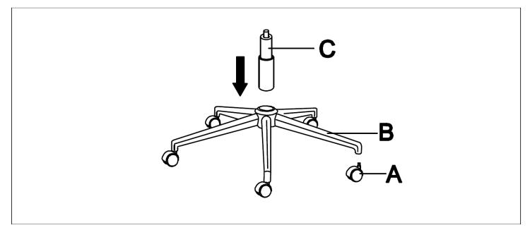
Place Star Base (B) upside down onto a padded, non-marring surface. Insert the 5 Casters (A) into the corresponding holes by pressing them firmly in place until fully seated. Turn the Star Base (B) assembly upright and then insert Gas Lift (C) into the center hole on the base as shown
