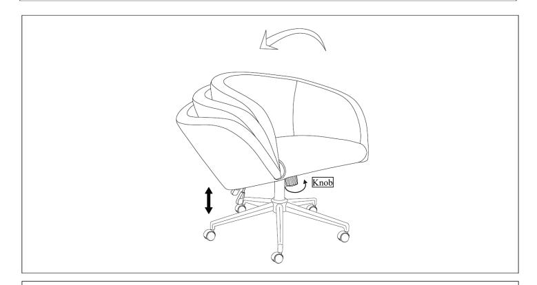
To lower the seat, life the lever upward while seated. To raise the seat, take your weight off the chair and pullthe lever. To increase or decrease the amount of recline, rotate the knob on the bottom of the seat. Adjust untilsatisfied
