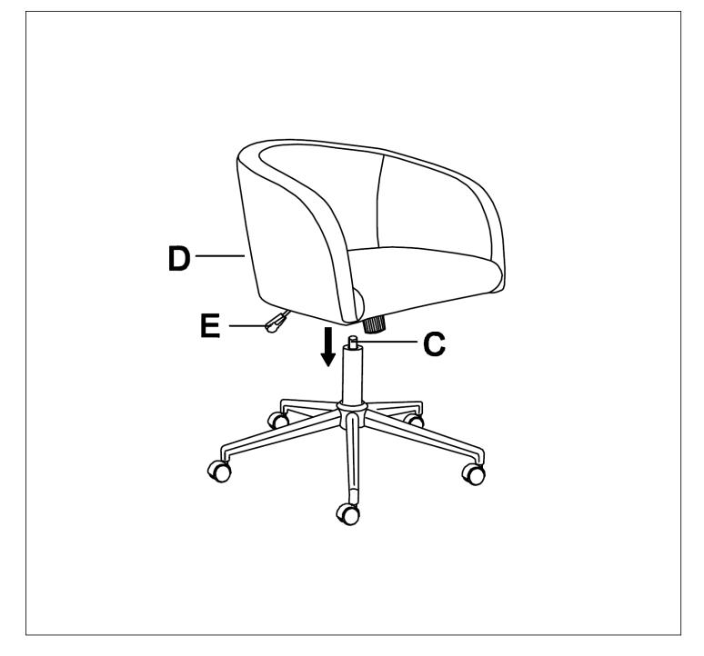
Carefully turn the Chair Top (D) assembly from Step 2 upright and position it over the top of the Gas Lift (C) as shown. Insert Gas Lift (C) into the center hole of Lift Mechanism (E). Press down firmly until the lift fully engages the center hole.
